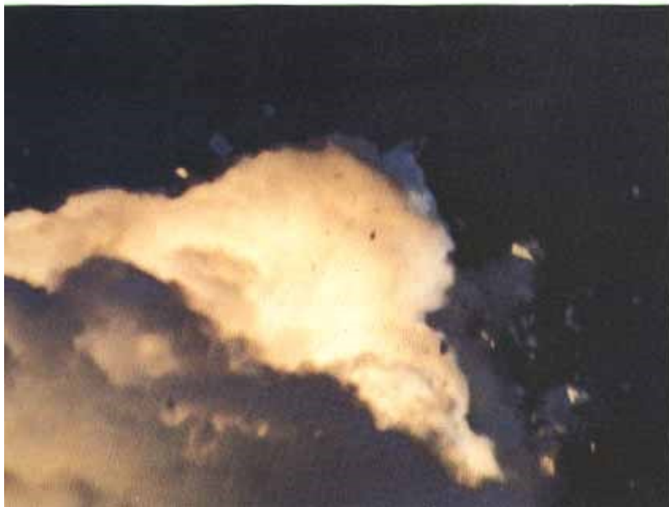
Fig. 14. At about 76 seconds, unidentifiable fragments of the Shuttle vehicle can be seen tumbling against a background of fire, smoke and vaporized propellants from the External Tank (left).
